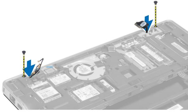
6. Remove the screws that secure the display assembly to the computer, and lift the display assembly from the computer.
