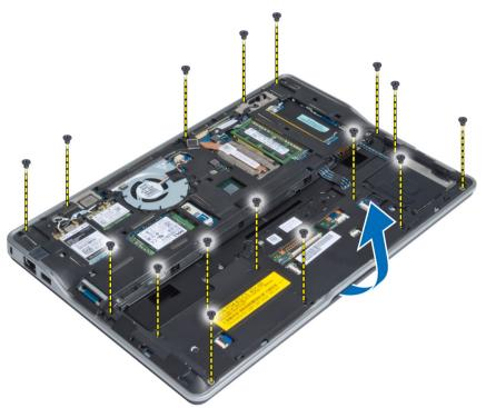
6. Press against the sections to release the palmrest assembly and remove it from the computer.
