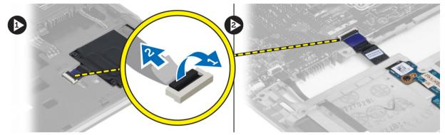
4. Remove the screws that secure the smart-card board in its place. Remove the smart-card cable from the routing channel and remove the smart-card from the computer.
