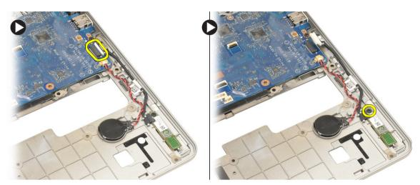
4. Remove the bluetooth card. Disconnect the cable from the card.
