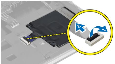
4. Remove the screws that secure the smart-card cage to the computer and remove it.
