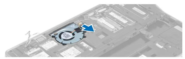
4. Disconnect the smart-card cable, hall-sensor cable and coin-cell battery cable.
