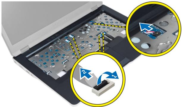
4. Remove the screws that secure the palmrest assembly to the computer.
